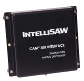
The TPD Air Interface combines temperature sensing and Partial Discharge detection. This broad band antenna is optimized for UHF radio detection methods for three distinct bands with center frequencies of 300 MHz, 600 MHz, and 1200 MHz while still providing capabilities for SAW sensor detection.
